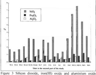
Figure 3 Silicon dioxide, iron(III) oxide and aluminium oxide content in samples from sites of the second phase of the study.
