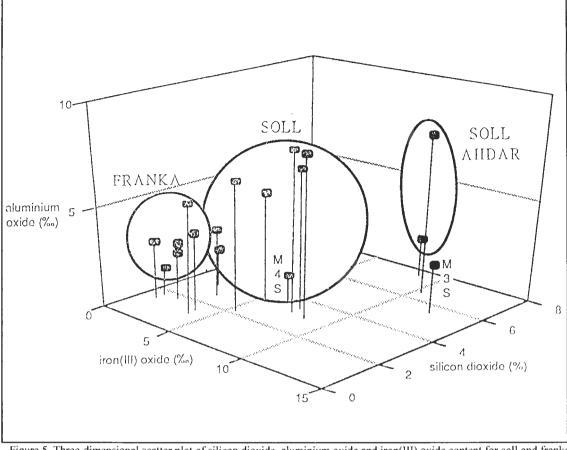
Figure 5. Three-dimensional scatter plot of silicon dioxide, aluminium oxide and iron(III) oxide content for soll and franka samples
